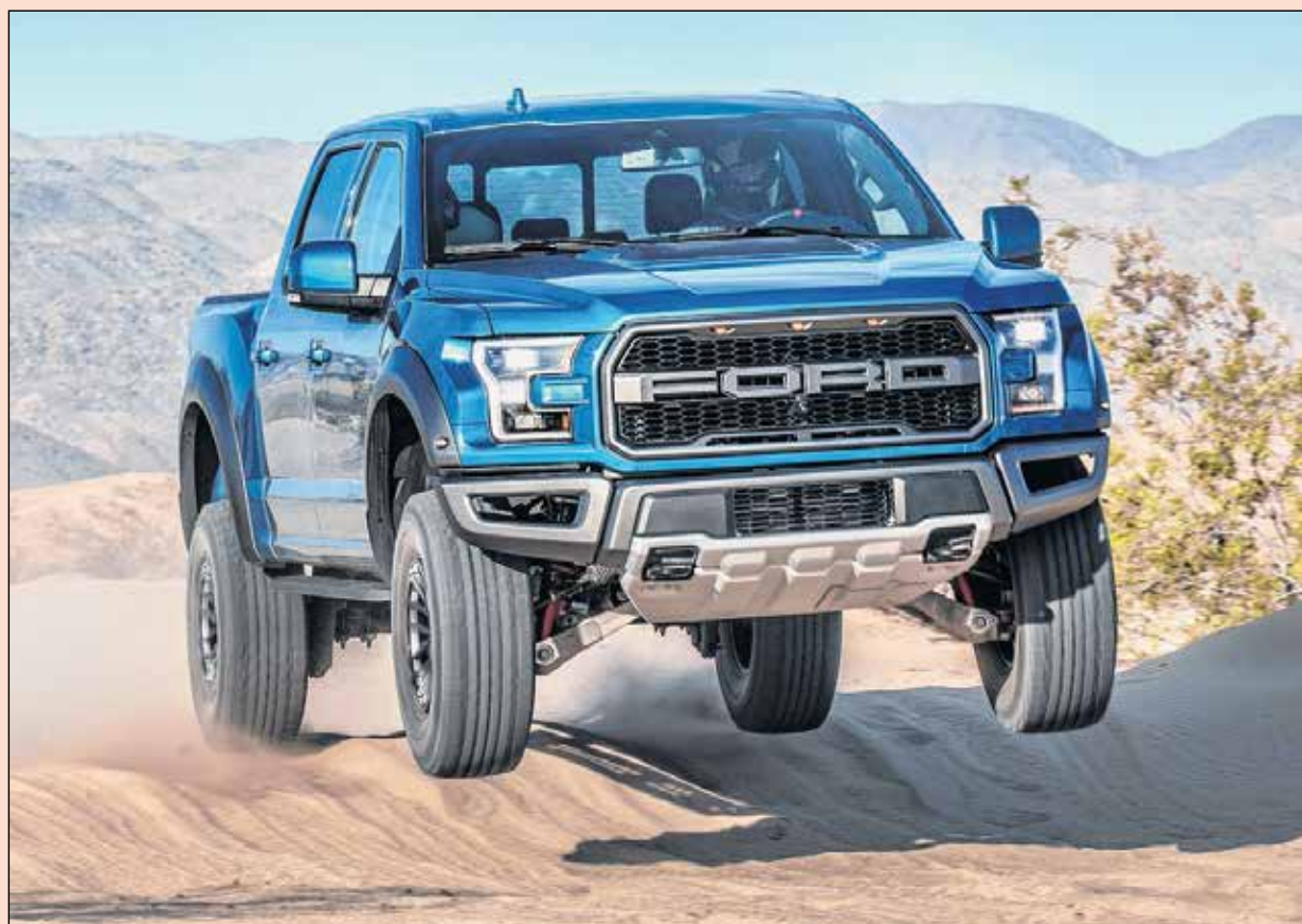
RAPTOR is the Ford F-150's high-performance pickup geared toward off-roading. Its 3.5L twin turbo, direct injection EcoBoost V6 generates 450 horses and 510 lb.-ft. of torque. Raptor is available in SuperCab and SuperCrew variants.
