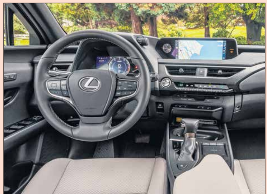
The 2019 Lexus UX 200's upscale interior features two-tone upholstery rather than monotonous. A console-mounted touchpad is the primary means of accessing many system controls, like climate, audio, navigation and general system settings.
