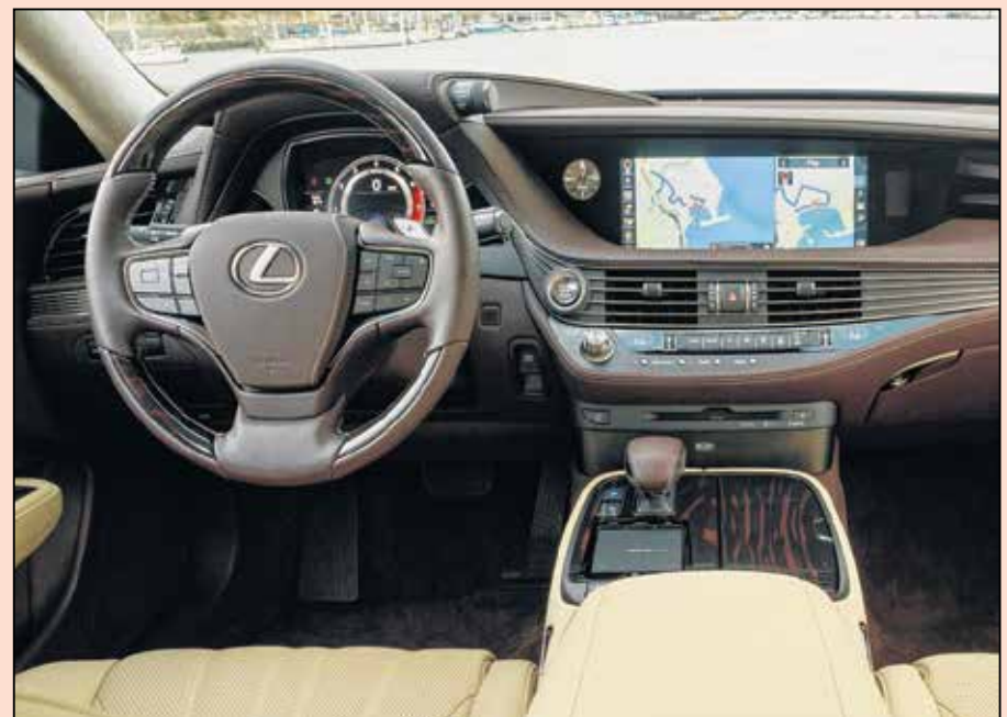
Many of the Lexus LS500's settings are absorbed into the 12.3-inch central display screen, accessed via touchpad on the center console. The process is inexact and distracting, and the system also buries items that should be more easily accessible
