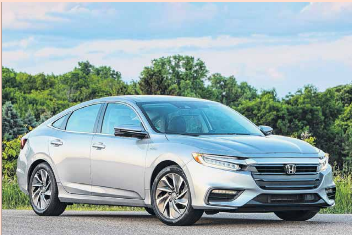
THE 2019 HONDA INSIGHT is propelled by a hybrid system of electric-drive motor and 1.5L, four-cylinder Atkinson cycle gas-powered engine (left). EPA mpg estimates are 51/45/48, though real-world figures may vary.
