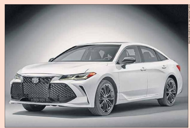
**THE 2019 AVALON** is Toyota's luxury sedan, offered with a 3.5L, six-cylinder engine (301 h.p.) or a hybrid version with a 2.5L Atkinson cycle four-cylinder (215 h.p.). Avalon is front-wheel-drive, with no AWD option.
