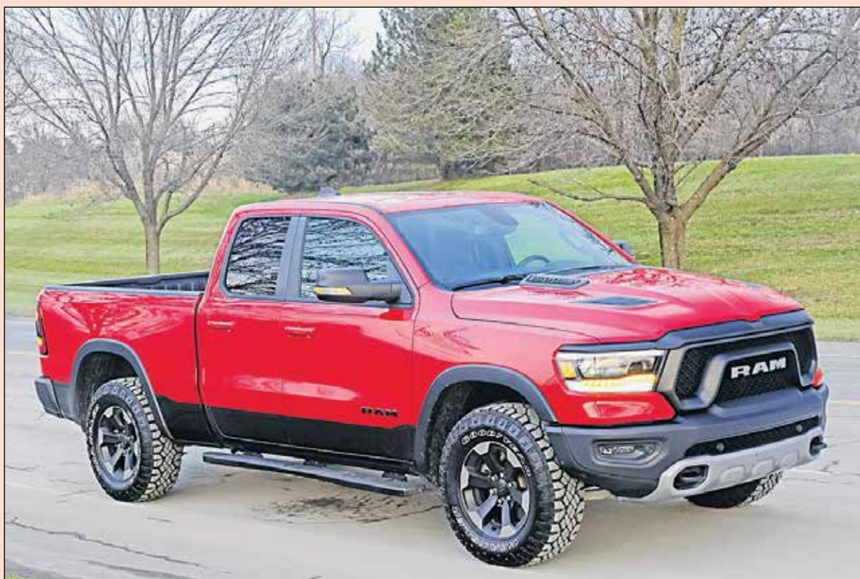
REBEL IS THE RAM 1500 MODEL with an off-road stance in mind. It sports 33-inch Goodyear Wrangler DuraTrac tires and a ground clearance of 8.7 inches. Engine options include a 3.6L V-6 and a 5.7L Hemi V-8.
