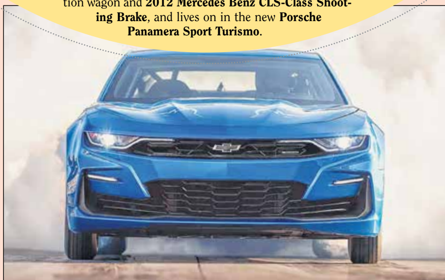
The electric eCOPO Camaro's 700 pounds of batteries create more than 700 horsepower.
