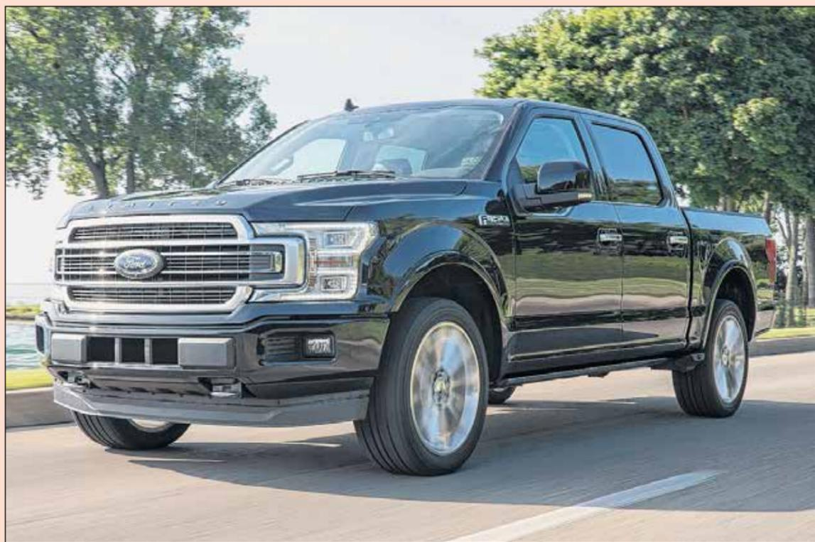
THE 2019 FORD F-150 comes in three different cab configurations: regular, SuperCab (smaller back doors) and SuperCrew (above) which is fitted with four full-size doors. It's also offered with six engine options and three bed lengths.
