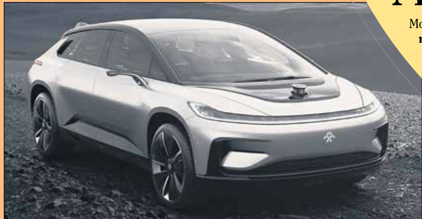
The Faraday FF 91 will have three electric motors that put out 1,050 horses.
