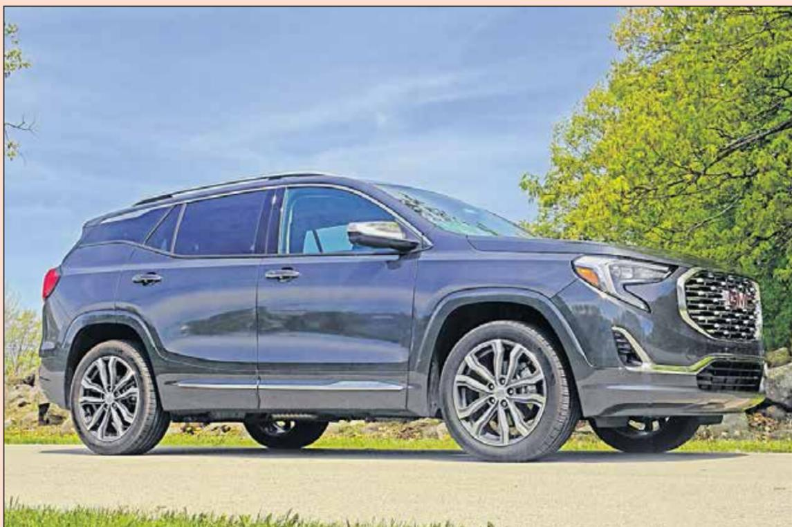
**THE 2018 GMC TERRAIN AWD DENALI** is GMC's midsize crossover, introduced in 2010 as a corporate cousin to the Chevy Equinox. The sole engine option for the Denali is the 2.0L four-cylinder, rated to tow up to 3,500 lb.
