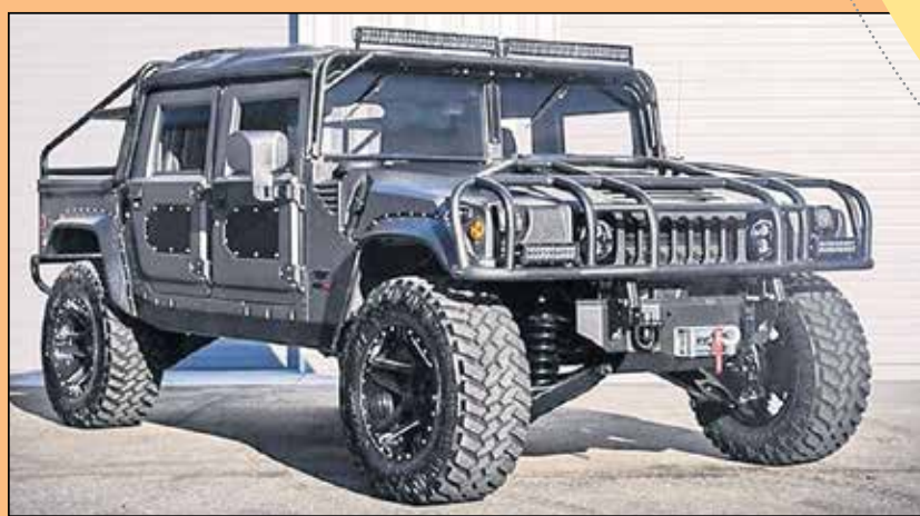
This modernized version of the Humvee from Mil-Spec Automotive will have aluminum body panels, 500 horsepower and 1,000 pound-feet of torque.
