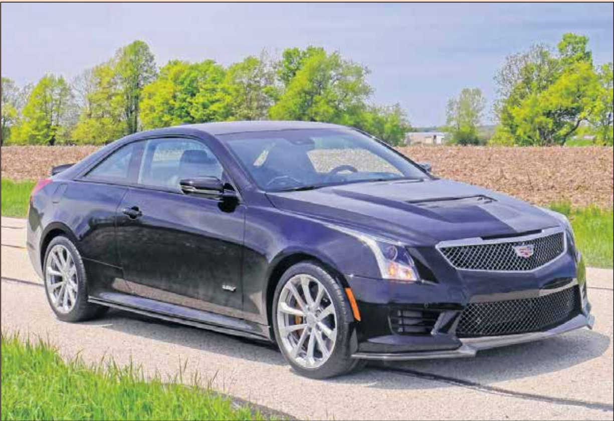
THE ATS-V is the performance version of Cadillac's entry level luxury compact, available in both sedan and coupe styles. It's powered by a twin-turbo 3.6L V-6 that generates a hefty 464 h.p., giving the ATS-V sub four-second 0 to 60 times.
