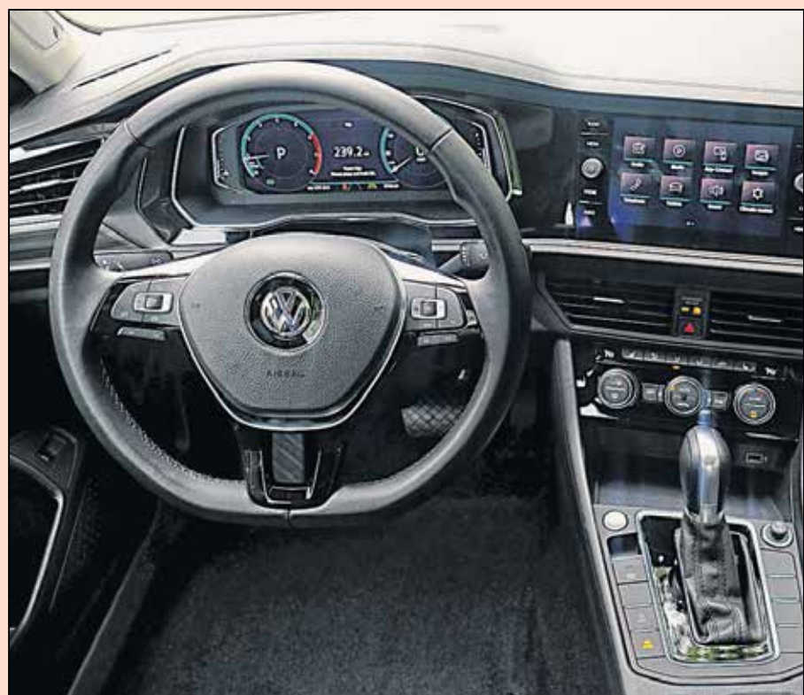
The interior of the 2019 Volkswagen Jetta has been redesigned. The SEL trim features a padded, textured dash above a 10¼-inch digital cockpit with 8-inch display.
