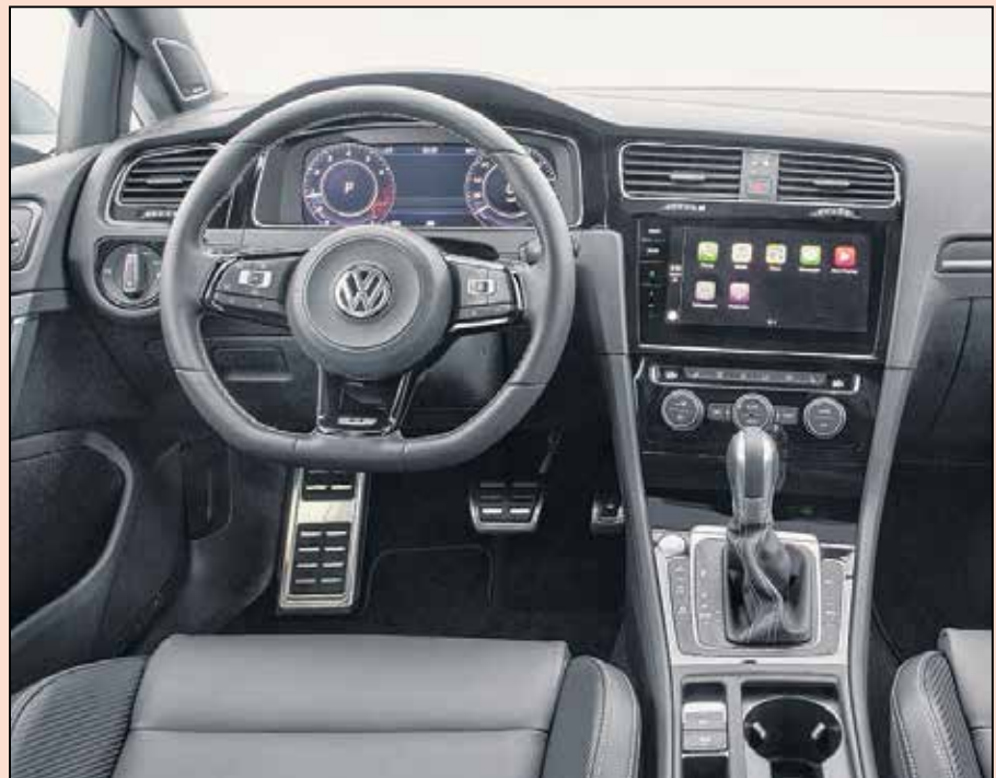
The 2018 Volkswagen Golf R's cockpit gains a notably larger (8-inch) touchscreen display and a customizable dashboard display that's Android Auto and Apple CarPlay compatible. Safety features include a pedestrian monitoring capability.
