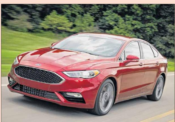
**FORD FUSION** is the American maker's midsize sedan, which carries over from 2017 largely unchanged, and is offered in five trim levels. The V6 Sport model is powered by a turbocharged, direct injected 2.7L rated at 325 h.p.
