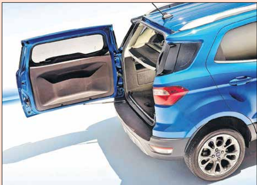
Unlike most vehicles in the subcompact crossover segment (which use a top-hinged liftgate), the Ford EcoSport uses a side-swinging door. The hinge on the left side allows for accessing the cargo bay while parked on the street without blocking the sidewalk.
