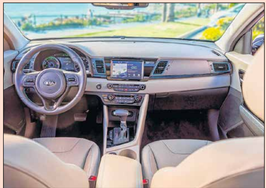
With a 7-inch display screen, Kia's UVO3 infotainment system includes voice recognition and is compatible with Android Auto and Apple CarPlay.
