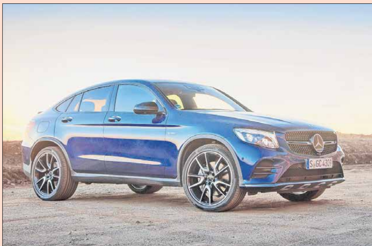
PHOTOS COURTESY OF THE MANUFACTURER THE 2018 MERCEDES-BENZ AMG GLC43 is a five-door hatchback based on the GLC crossover chassis. The high performance version's AMG-tuned 3.0L biturbo V-6 (left) is paired with an enhanced 9G-tronic automatic transmission.
