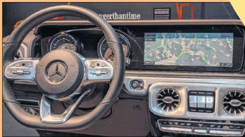
The Mercedes-Benz G-Wagon's multifunction steering wheel with paddle shift switches is shared with the revised S-Class.
