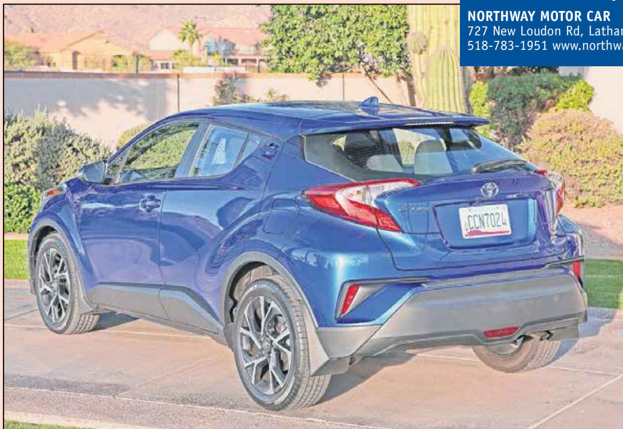
The front-drive, two-door compact Toyota C-HR shares the same unibody platform as the Prius and Camry.
