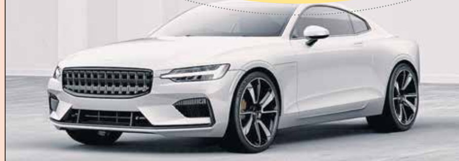
The Polestar 1 foreshadows a halo model from Volvo with a body made mostly of carbon fiber. The 600-hp hybrid sports coupe has a 93-mile EV range.
