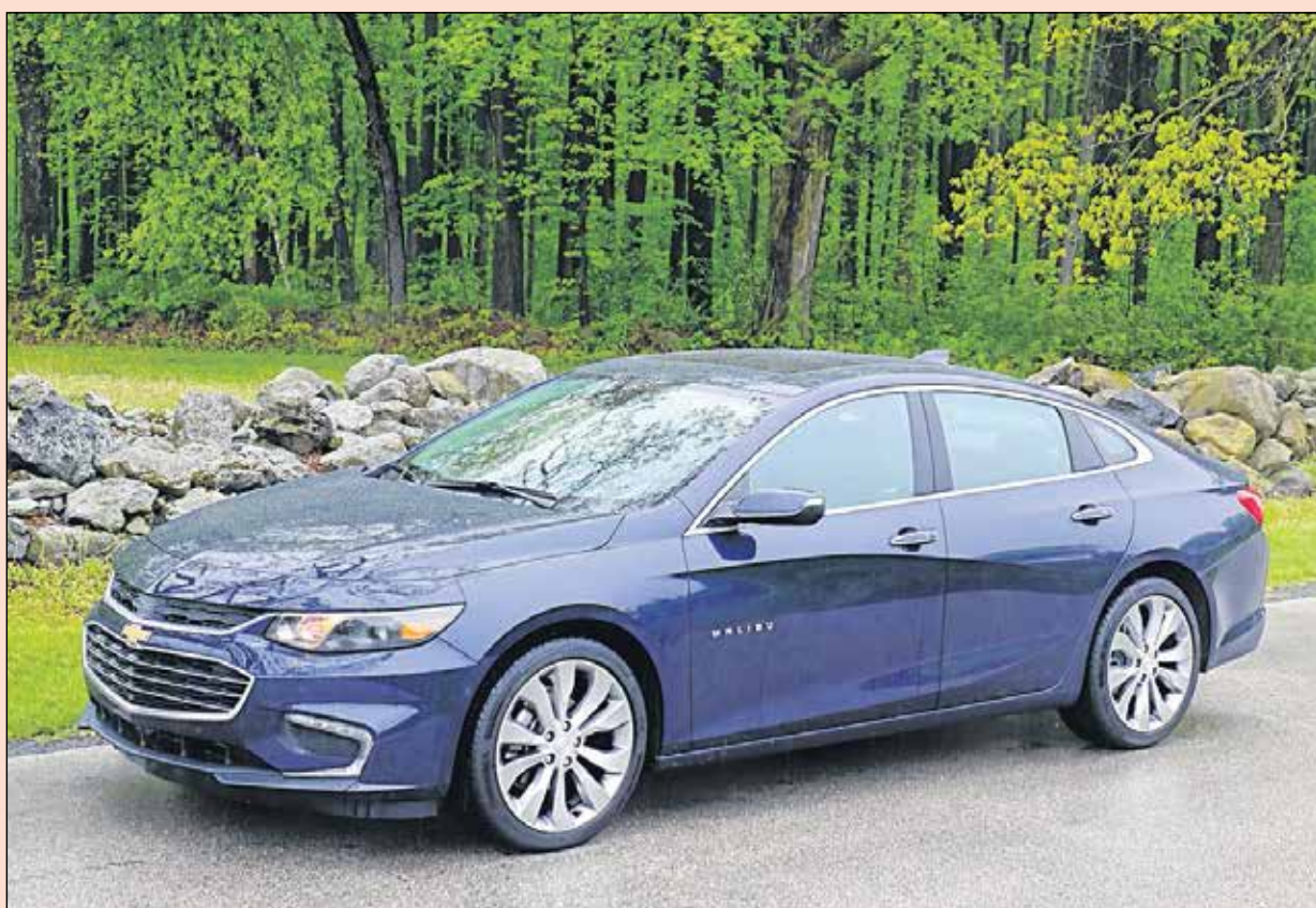
THE 2018 MALIBU is Chevrolet's offering in the midsize sedan segment, slotted between Impala and Cruze. It's powered by a turbocharged 1.5L four-cylinder or, in the Premium level trim, a 2.0L four (left).
