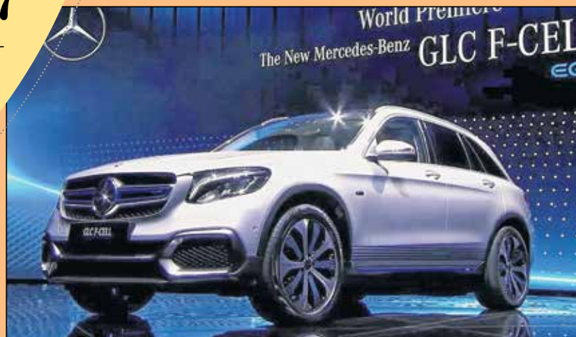
Shown at last month's Frankfurt Auto Show, the Mercedes-Benz GLC F-Cell is the world's first plug-in fuel-cell vehicle. Headed for pre-production, the GLC F-Cell has a range of 301 miles from just 9.7 lbs. of hydrogen and a 13.8-kWh battery.
