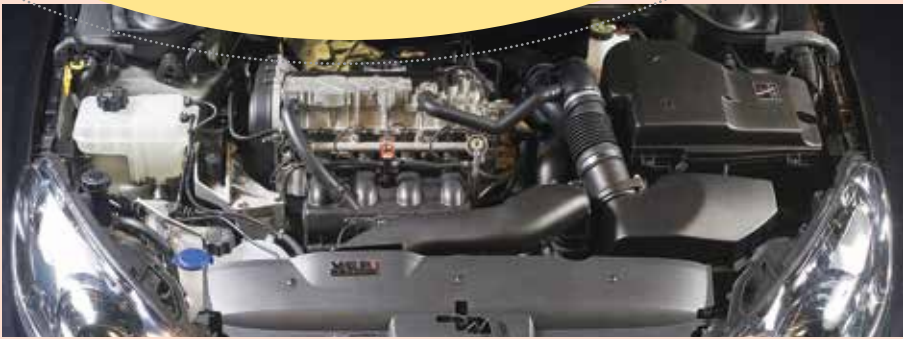
At the 2016 Paris auto show, Nissan showed off the Infiniti's QX Sport Inspiration concept, most notable for its production-ready, variable-compression-ratio four-cylinder engine (VC-T) that offers more fuel-efficiency and lower emissions. It will go into the next QX50 crossover in 2018.
