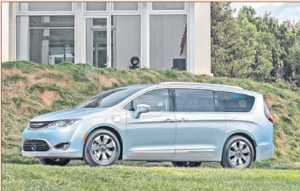
Chrysler's newest minivan is the hybrid version of the Pacifica, which replaced the Town & Country. It offers a 30-mile range on a single charge of its 16-kW battery pack, while a 3.6L V-6 gas engine extends the overall range to 530 miles.
