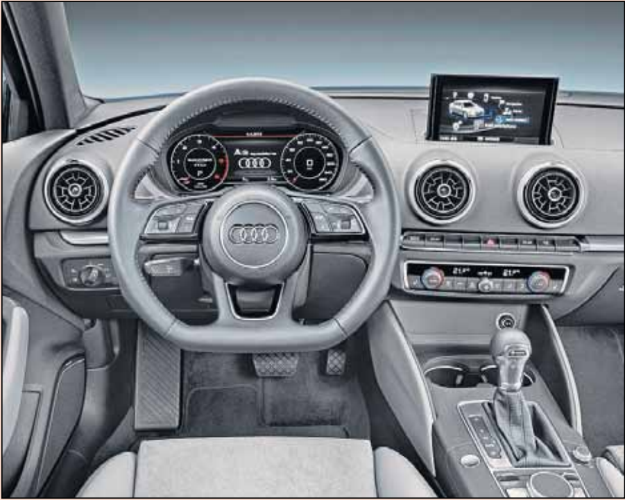
The overall look and feel of the Audi A3's interior is handsome and well finished. HVAC functions are controlled by a trio of dials, while other functions are by other switches. A think 7-inch color display retracts flush with the dashboard surface.
