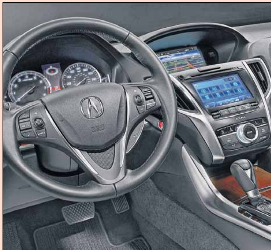
The 2016 Acura TLX's main dash cluster is clean and legible, with HVAC and sound systems accessed by conventional controls while others are absorbed into one of the two main, dual-tiered touchscreens. Shortcuts are also available on the steering wheel.
